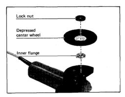
To tighten the lock nut, hold the spindle with the wrench so that it cannot revolve, then use the lock nut wrench and securely tighten clockwise.
